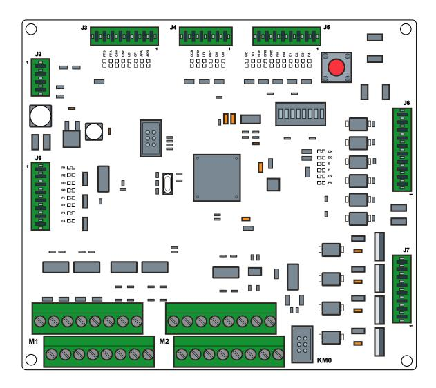
Inspection control is actuated by switching the respective control panel switch from "NOR" to "ISP"; the RM relay will excite and send the inspection control active signal to board input J5/2 (RM), following which the board will check the safety chain and then activate the contactors by setting the up or down direction depending on the commands received and check that they excite/de-excite accordingly. There are two ways to move the car in inspection mode:
